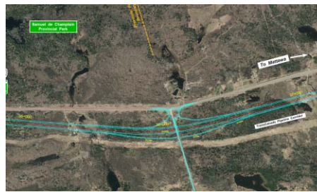
Alternative 2 Diamond – Roundabout Configuration
