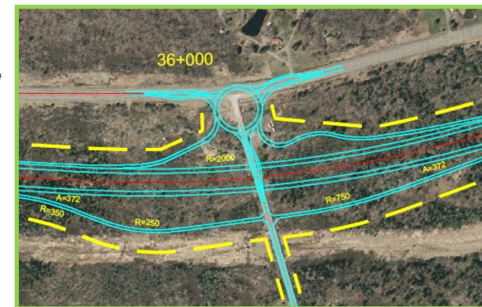
Boundary Road Interchange Diamond - Roundabout Configuration
